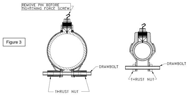
5. Hold the PLIDCO Smith+Clamp firmly in position until the drawbolt and thrust nuts are tightened to the torque value indicated in Chart A.
