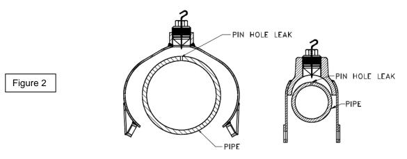
3. Loosely assemble the PLIDCO Smith+Clamp on the pipe next to the leak. Insert the drawbolt but do not tighten.
